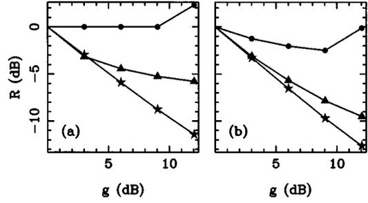
FIG. 1. Noise figure vs gain  $g$  (integer powers of 2) for input phase-coherent state (stars), coherent state (circles), and squeezed state (triangles) with  $\langle\hat{n}\rangle_{in}=40$  and  $\varphi=0.05$  for all states (the squeezed state has 2.6 squeezing photons: see [18]). (a): ideal detection. (b): heterodyne detection.
