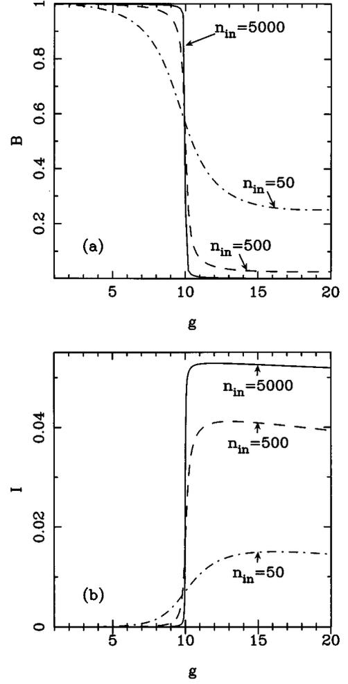
FIG. 3. Bit-error rate (a) and mutual information (b) vs gain  $g$  for phase-coherent states with input number of photons  $\langle \hat{n} \rangle_{in} = 50, 500, 5000$ . The phase shift is  $\varphi = 0.05$ , whereas the threshold phase is  $\varphi_s = 0.5$ . For the mutual information a probability  $p_1 = 0.01$  has been used (rare events).
