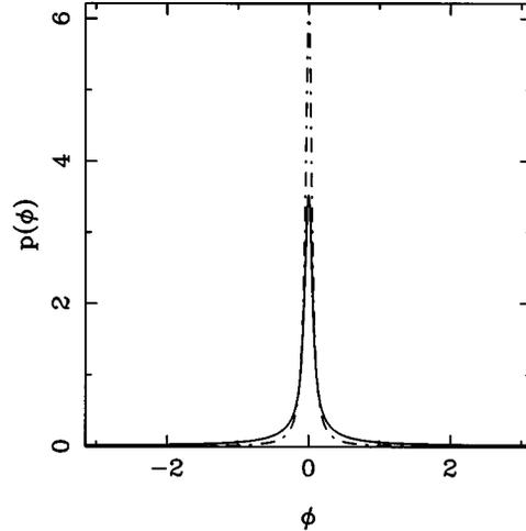
FIG. 5. Phase probability distribution of a phase-coherent state compared with the probability of a state achieved using a PIA and a sum frequency up converter in series (the sharper probability refers to the ideal state). The resulting average photon number is  $\langle \hat{n} \rangle = 9.26$ .
