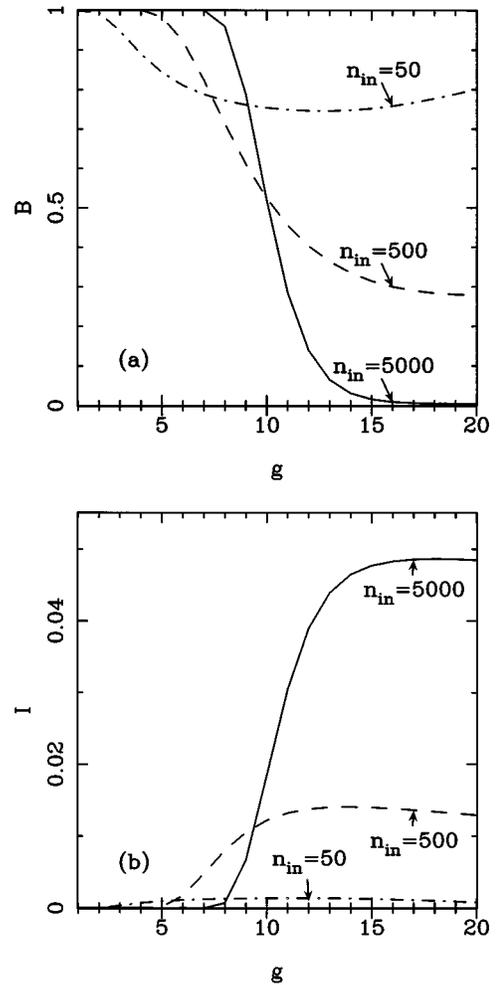
FIG. 4. Bit-error rate (a) and mutual information (b) vs gain  $g$  for coherent states and heterodyne detection (same values of parameters as in Fig. 3).
