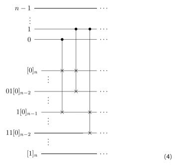
In words, for k = 0 to n - 1 the circuit does the following: insert  $2^k$  control-swaps controlled by the (k + 1)th control qubit and swapping system qubit  $[s]_k[0]_{n-k}$  with system qubit  $[s]_k1[0]_{n-k-1}$  for every k-bit string  $[s]_k$ .
