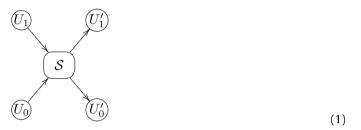
where  $\mathcal S$  represents the QS having two inputs and two outputs,  $U_0$  and  $U_1$  denote the two input unitary channels, and  $U_0'$  and  $U_1'$  are the two output ones, which are either  $U_0'=U_0$  and  $U_1'=U_1$  or  $U_0'=U_1$  and  $U_1'=U_0$ , depending on the state  $|0\rangle$  or  $|1\rangle$  of a control qubit s (not represented). In formula
