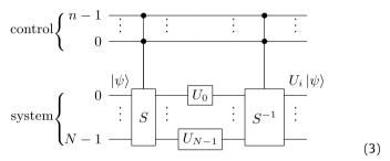
In the circuit, the system register is prepared in the state  $|\psi\rangle \otimes |0\rangle^{N-1}$  and the control in the state  $|[i]_n\rangle$ . This will output the state  $U_i|\psi\rangle$  on the first system qubit. For this purpose one first operates an n-controlled swap S, then each system qubit i undergoes  $U_i$ , and finally an inverse n-controlled swap  $S^{-1}$  is made. The n-controlled swap is achieved by the following circuit:
