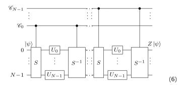
where  $Z=U_{i_{(N)}}\dots U_{i_{(1)}}$  denotes the programmed disposition of unitaries, and  $\mathscr{C}_i$   $(i=1,\dots,N)$  denote a control register made of n qubits. The circuit is just the juxtaposition of N copies of circuit (3),  $\mathcal{C}_i$  being the control system of the *i*the circuit.
