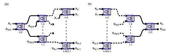
FIG. 3. (a) A network of N-1 quantum switches which multiplexes an input photonic signal from the  $x_0$  spatial mode into one of N spatial modes. (b) A network of N-1 quantum switches which demultiplexes N spatial modes of a photonic signal into a single spatial mode  $(x_0)$ .
