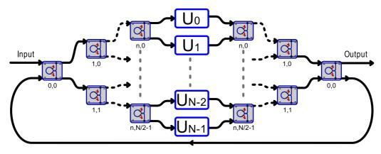
FIG. 4. An optical device which simulates N-switch using 2N-2 quantum switches and N physical quantum operators. Because the behavior of the quantum switches is governed by a predetermined pattern of optical control pulses, the time at which a photonic signal is input to the device can be mapped to an order in which the photon passes through the quantum operators.
